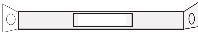
BASE PLATE W/ADHESIVE BACKING AND BENDS AT ENDS WITH A HOLE FOR SECURITY CABLE TO PASS THROUGH
